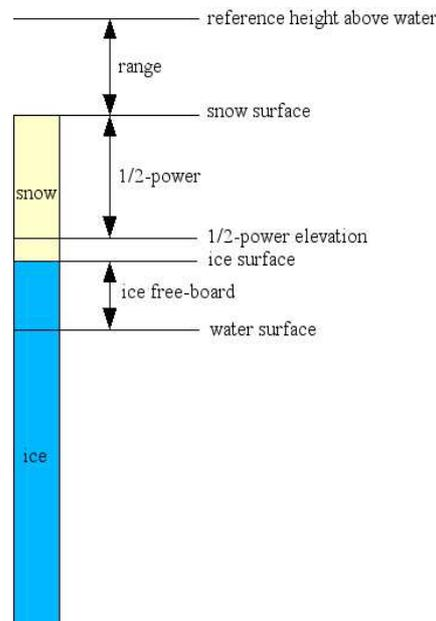
Fig.1. Showing the definition of terms used in the simulations.
