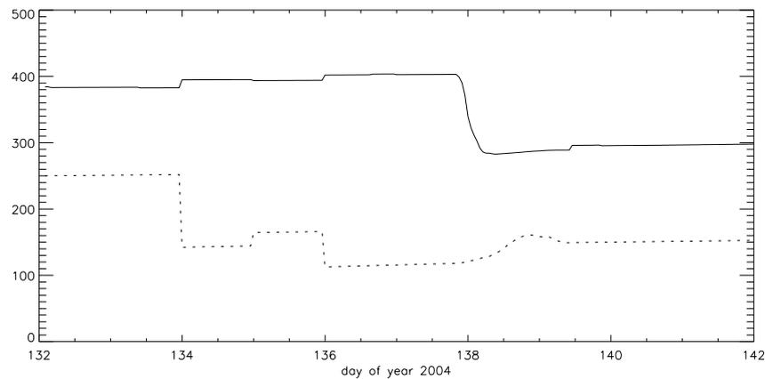
Fig.6. (continued from fig. 5). The range +  $\frac{1}{2}$  - power time [ $1 \times 10^{-11}$ s] (solid line) and the upper snow layer density [ $\text{kg/m}^3$ ] (dotted line) is simulated using a modified meteorological record from the GreenIce camp in the Lincoln Sea May 2004 and the multiyear ice profile in Appendix I.
