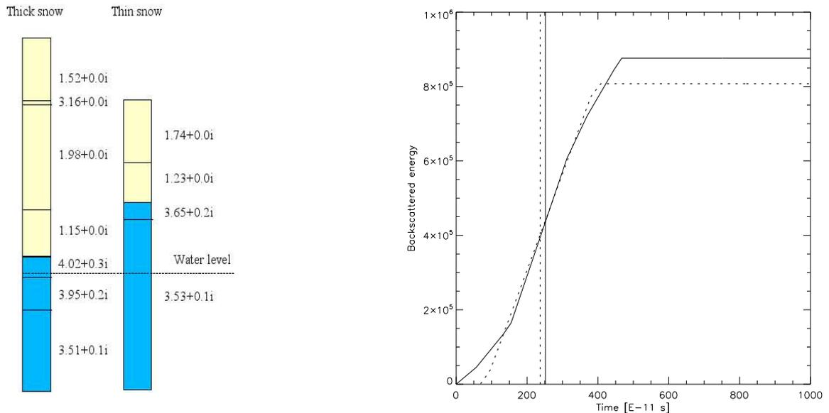
Fig. 2a. (left) The permittivity of the snow and ice layers in the thin and thick first-year ice profiles
