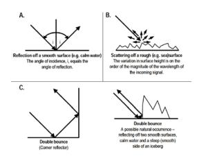
**Figure 1.** Radar signals - reflection and scattering off at the boundary of different surface types.
